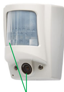
Infrared PIR detector activates the camera
